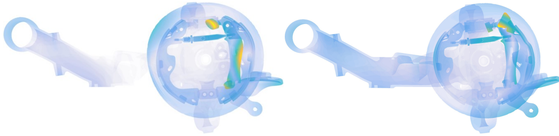
Figure 12 : Expansion result for the two extracted experimental shapes from the limit cycle measurements.
