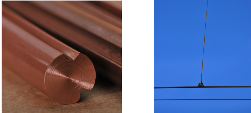
Figure 1.2: Contact wire (CW) (left) and dropper (right)
