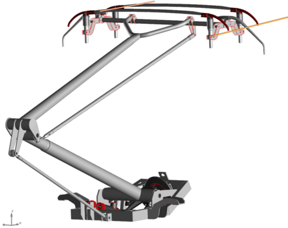
Figure 5 – Multibody pantograph: overhead crossing simulation
