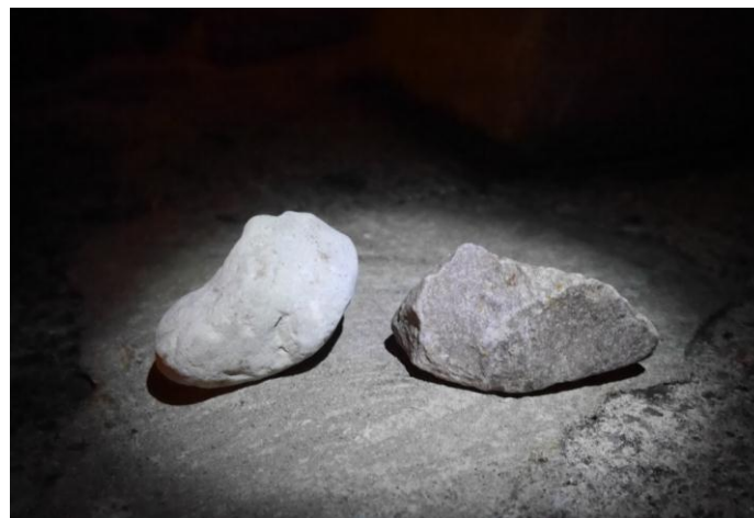
Figure 10: Ballast particles of Chauconin zone. Left particle is from transition zone, right particle is from current ballast track
