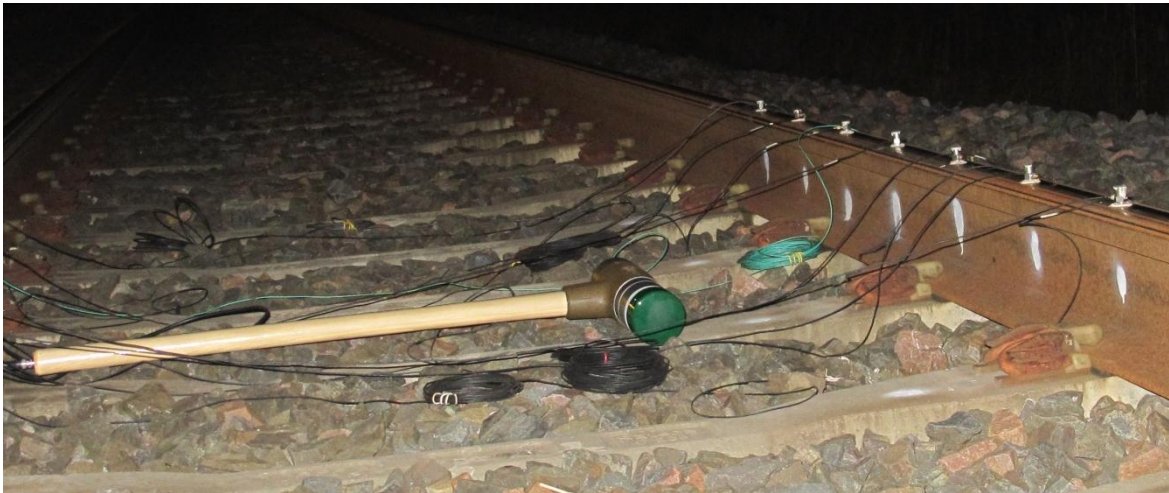
Figure 2: Experimental device for receptance test in Chauconin
