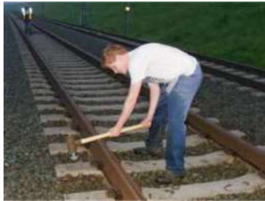
Figure 2: Hammer impact on rail, from (Verbraken et al.,2011)
