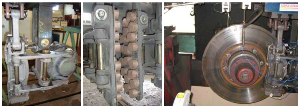
FIGURE 1: The TGV disc-brake system : "caliper-type" structure (left), pads fixed into the caliper (center), brake assembly on the test bench (right)
