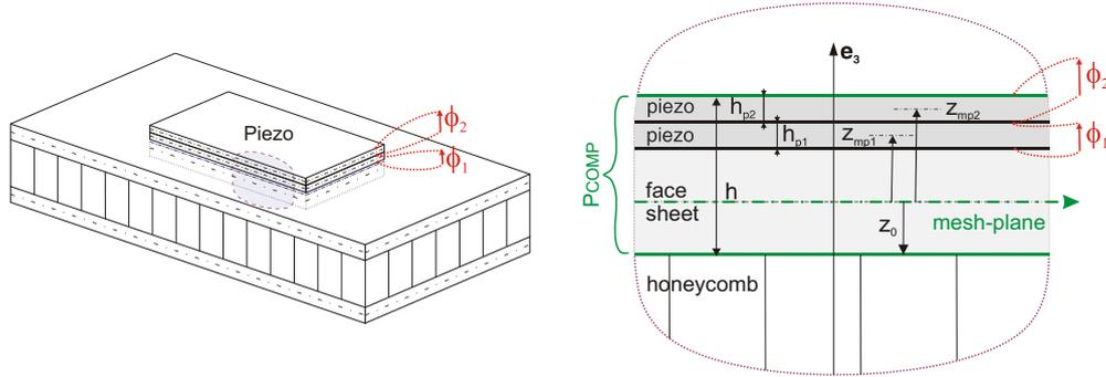
**Figure 5.5:** Modeling of sandwich beam with piezoelectric layers
