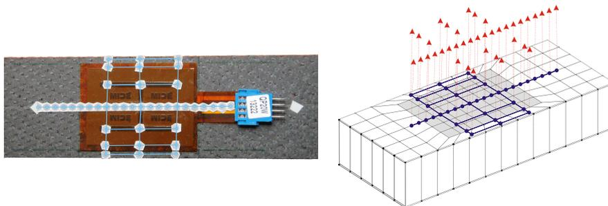
Figure 5.23: Measurement locations for the modal test focusing on the patch behavior
