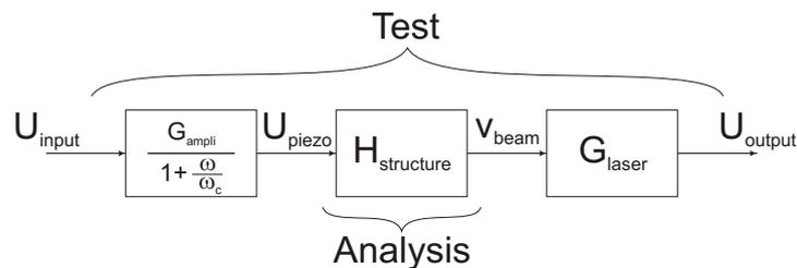
**Figure 5.3:** *Functional representation of the measurement loop*
