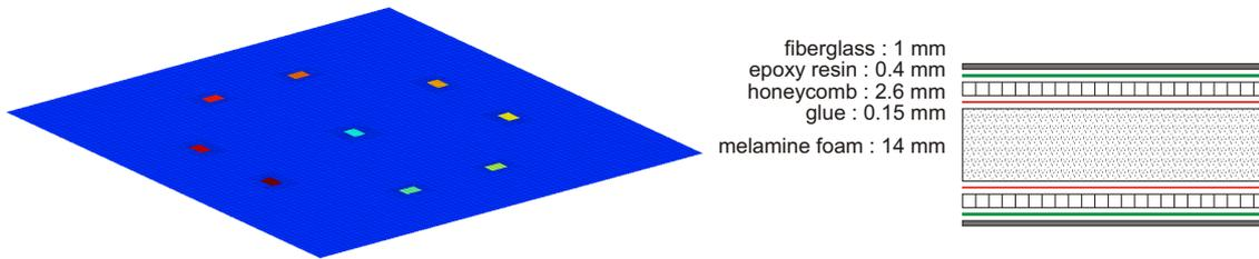
**Figure 5.35:** Trim panel used in VASCo mock-up. Left: patches localization. Right: description of sandwich layers
