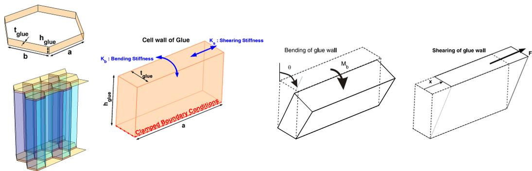
**Figure 3.15:** Parameterization and stress on glue element
