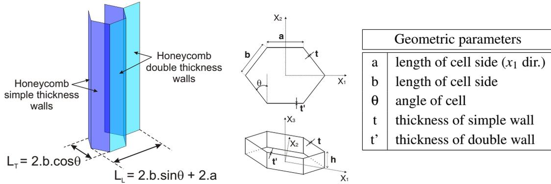
Figure 3.11: Definition of honeycomb core geometric parameters
