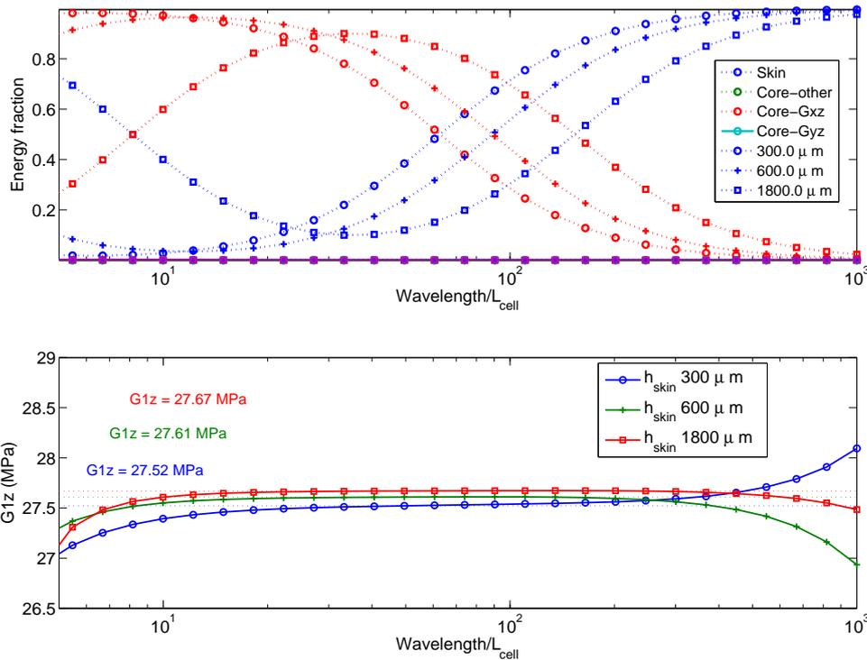
**Figure 3.30:** Top: Energy contribution of constituents for bending along x-direction - Face sheet thickness:  $h_{f_0}/2$ ,  $h_{f_0}$  and  $3 * h_{f_0}$ . Bottom: Estimation of  $G_{xz}^*$  associated with no error - Core mass correction +0.75%
