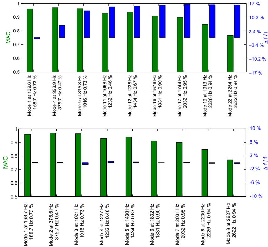
**Figure 4.24:** Test/analysis correlation with  $G_{yz}^* = 18 \text{ MPa}$  (top) and updated  $G_{yz}^*$  (bottom) at  $25^\circ \text{C}$  - MAC and frequency error for bending modes
