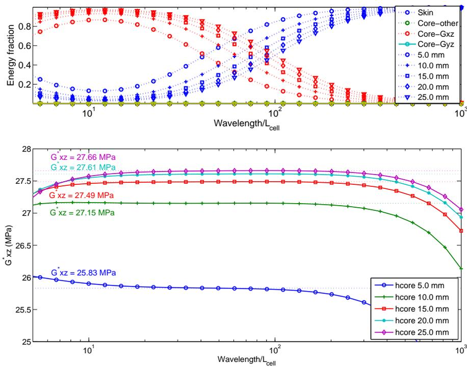
**Figure 3.32:** Top: Energy contribution of constituents for bending along x-direction - Core thickness: 5, 10, 15, 20 and 25mm. Bottom: Estimation of  $G_{xz}^*$  associated with no error - Core mass correction +0.75%
