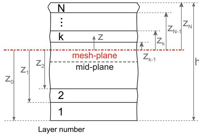
**Figure 2.3:** Geometry of an  $N$ -layered laminate
