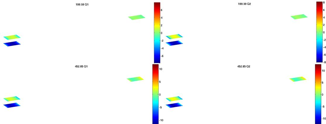
**Figure 5.17:** Bending response at 199.39 Hz (top) and 452.85 Hz (bottom) for membrane actuation (Piezo 3). Charge in the top Q2 (shown right) and bottom Q1 (shown left) electrodes shown with the same scale
