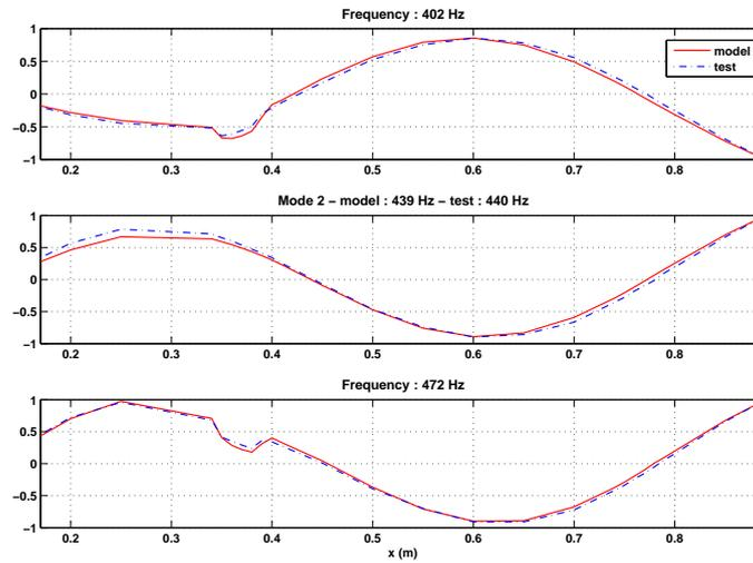
Figure 5.22: Test and simulation deflection shape comparison
