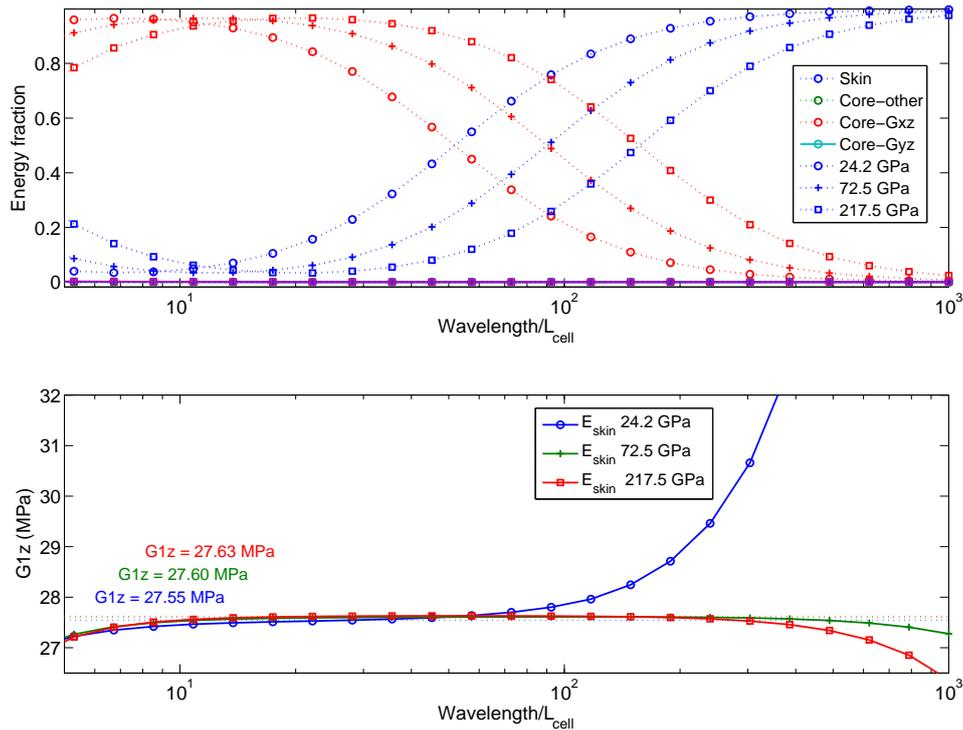
**Figure 3.29:** Top: Energy contribution of constituents for bending along  $x$ -direction - Face sheet Young modulus:  $E_{f_0}/3$ ,  $E_{f_0}$  and  $3E_{f_0}$ . Bottom: Estimation of  $G_{xz}^*$  associated with no error - Core mass correction +0.75%
