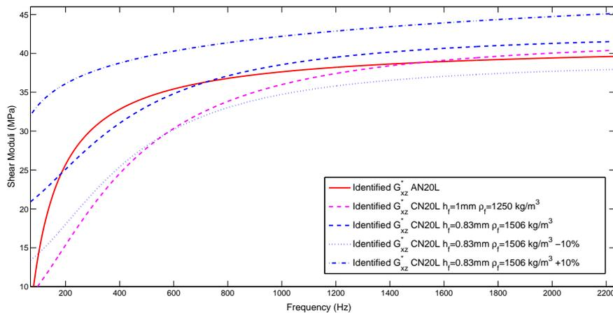
**Figure 4.26:** Influence of skins thickness on the viscoelastic law of experimental transverse shear modulus  $G_{xz}^*$  for CN20L beam,  $h_f = 1\text{mm}$  and  $0.83\text{mm}$ , compared to  $G_{xz}^*$  for AN20L beam
