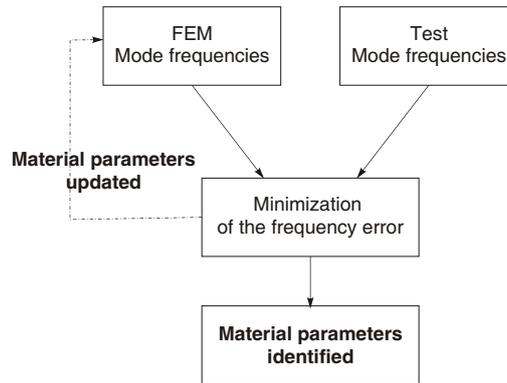
**Figure 4.19:** Process of parameter estimation by updating
