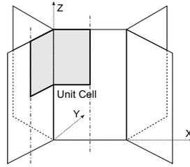
**Figure 2.9:** Grediac and Meraghni's representative unit of honeycomb for numerical estimation
