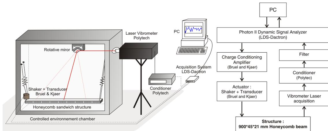
Figure 4.3: Left: Experimental setup. Right: Acquisition chain.
