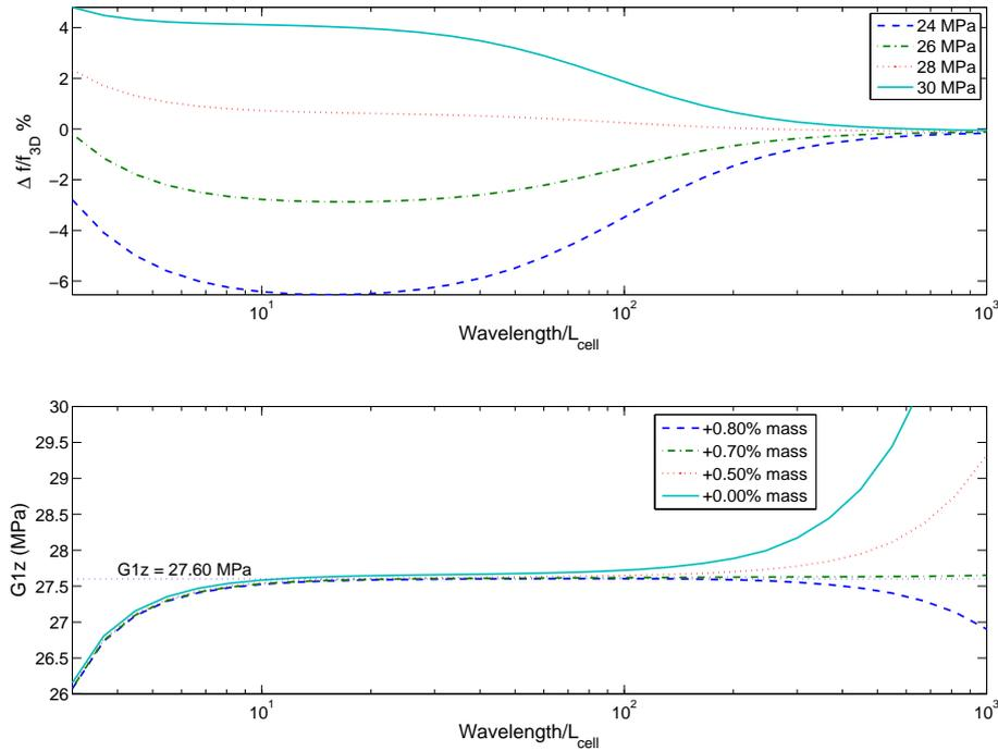
**Figure 3.20:** Top: error on the first periodic bending mode frequency for various values of  $G_{xz}^*$ . Bottom: Estimation of  $G_{xz}^*$  associated with no error. Detailed 3D model with 1 element per cell wall
