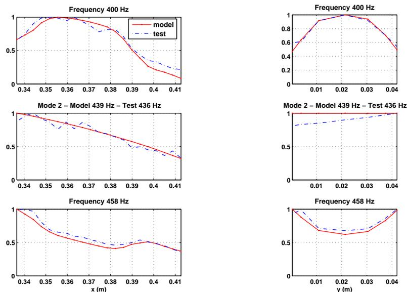
**Figure 5.25:** Local blister shape comparison on the x and y axes.
