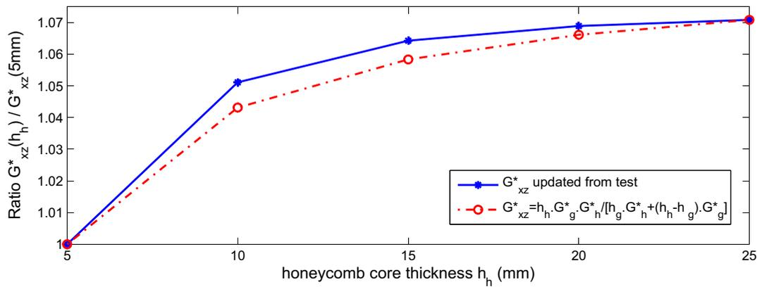
**Figure 3.33:** Ratio  $G_{xz}^*(h_h) / G_{xz}^*(5mm)$  for  $G_{xz}^*$  estimated through numerical homogenization and calculated from  $G_g^*$  and  $G_h^*$  (3.30)
