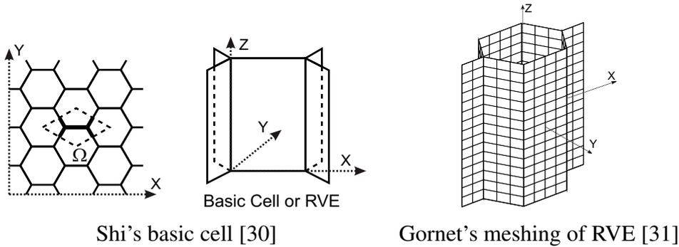
**Figure 2.11:** Representative Volume Element for homogenization theory
