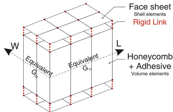
**Figure 3.4:** Geometry of the Shell Volume Shell (SVS) model
