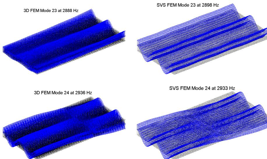
**Figure 3.28:** Example of SVS/3D FEM modes poorly correlated (23<sup>rd</sup>, 24<sup>th</sup>)
