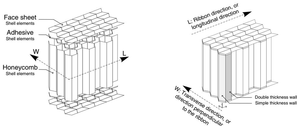
**Figure 3.2:** Definition of the 3D finite element model
