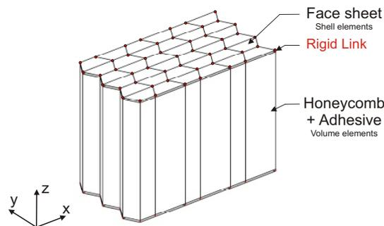
**Figure 3.18:** SVS model with skin geometry of the 3D model
