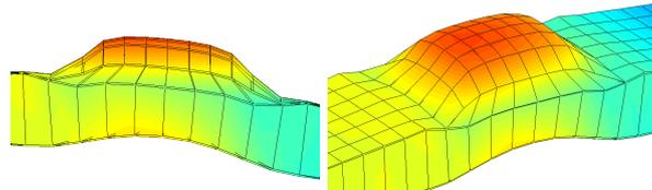
**Figure 5.26:** *Blister of piezoelectric actuator. Simulated response at 375 Hz*
