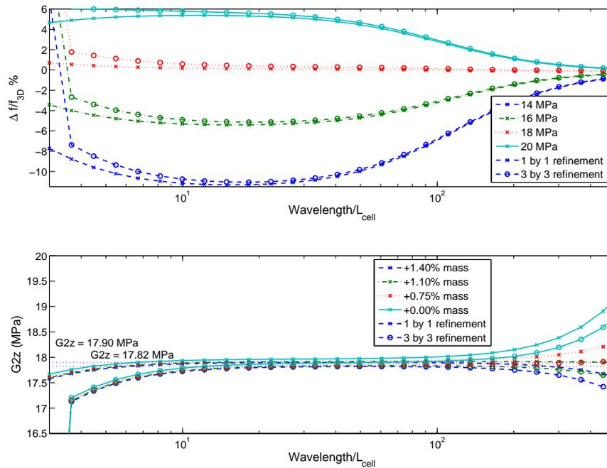
**Figure 3.24:** Top: error on frequency of the first periodic bending mode for various values of  $G_{yz}^*$ . Bottom: Estimation of  $G_{yz}^*$  associated with no error. Superposition for 3 elements and 1 element per cell
