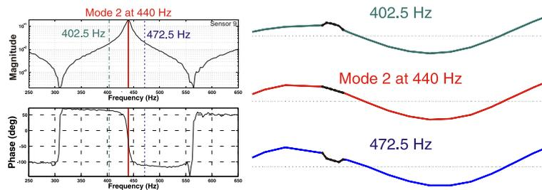
**Figure 5.19:** *Left : Transfer from patch 1 to displacement at the middle of the patch around the frequency of test mode 2. Right : shape before, at, and after resonance. Carbon/Nomex honeycomb core beam*
