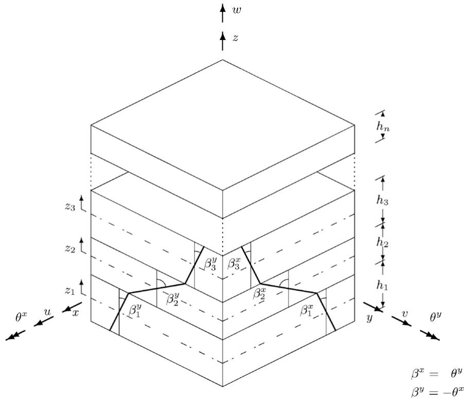
**Figure 2.6:** Layerwise theory - Moreira's kinematic model [1]
