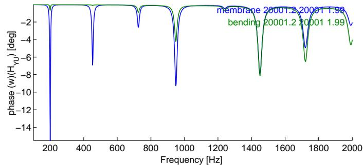
**Figure 5.14:** Phase of impedance (transfer from tension to charge) at Piezo 1 - Cabling 1 (membrane) and Cabling 2 (bending)
