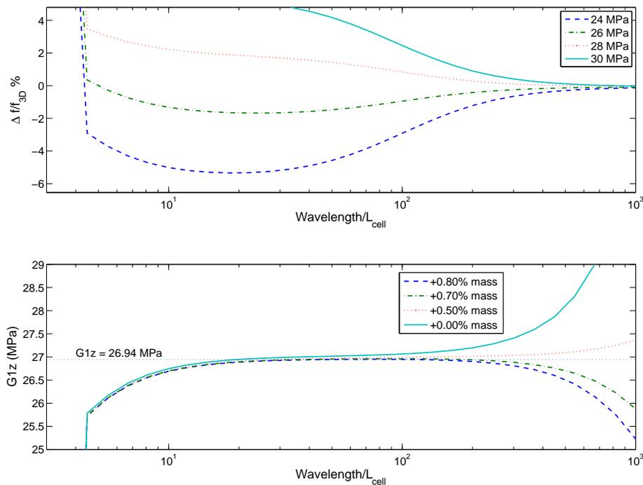
**Figure 3.19:** *Top: error on the first periodic bending mode frequency for various values of  $G_{xz}^*$ . Bottom: Estimation of  $G_{xz}^*$  associated with no error. Detailed 3D model with 3 by 3 refinement (curves correspond to +0.8% to 0% mass)*
