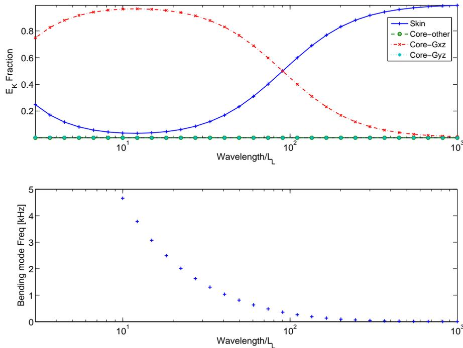
**Figure 3.13:** Top: Energy contribution of constituents, SVS model, bending along  $x$ -direction. Bottom: Frequency of first periodic mode along  $x$ -direction
