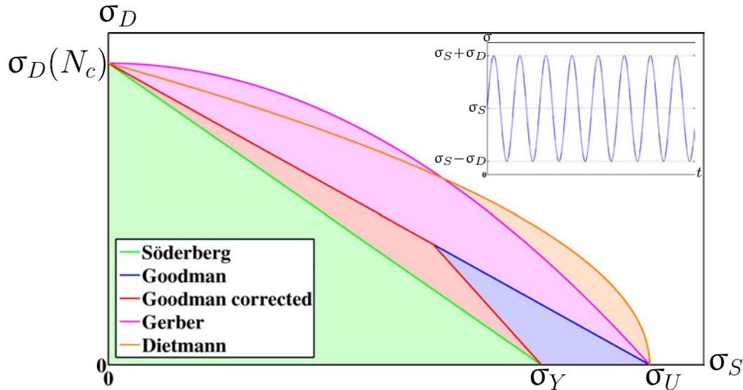
Figure 5: Haigh diagram with the approximate limit curves and safe areas (positive stresses only) —  $\sigma_S$ : static stress,  $\sigma_D$ : dynamic stress,  $\sigma_Y$ : yield stress,  $\sigma_U$ : ultimate stress and  $N_c$ : number of cycles
