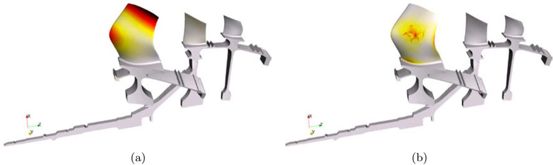
Figure 2.30: Mono-harmonic eigensolution localized to disk  $\mathcal{D}^1$  with  $\delta = 4$  at  $f = 8.63$ : (a) amplitude of the displacement and (b) density of strain energy — Blade shape is 2F [3SHP]
