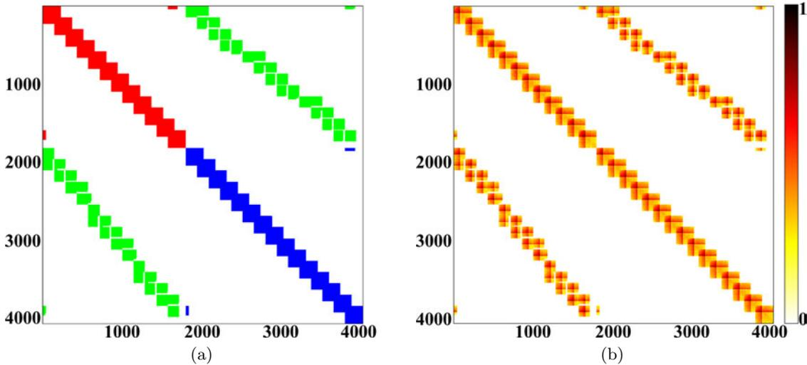
Figure 2.26: Reduced stiffness matrix  $[K_M]$  (a) global shape: (■) blocks of disk  $\mathcal{D}^1$ , (■) blocks of disk  $\mathcal{D}^2$  and (■) blocks of ring  $\mathcal{R}$ , and (b) actual matrix (ACAD model with 12 and 15 sectors)
