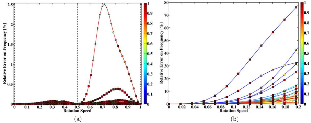
Figure 3.13: Relative error on frequency and modeshape correlation for a multi-model Craig-Chang-Martinez reduction techniques built at (a)  $\Omega \in \{0, 0.5, 10\}$  and (b)  $\Omega \in \{0\}$  — The color bars refer to the modeshape correlation [BB]
