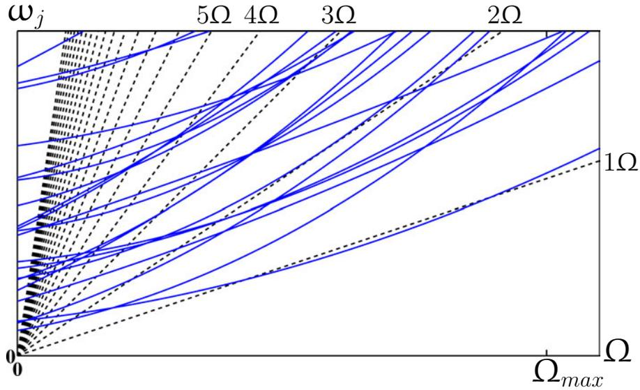
Figure 4: Campbell diagram with (– –) engine-order excitation lines
