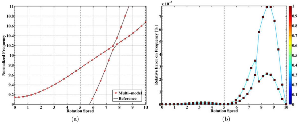
Figure 3.7: (a) Campbell diagram for  $\delta = 1$  and (b) relative error on frequency restricted to mode pairs 6 and 7 for a multi-model built at  $\Omega \in \{0, 5, 10\}$  — The color bar refers to the modeshape correlation [HEBD]
