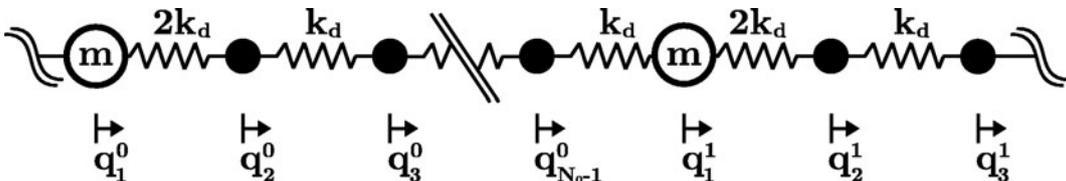
Figure 1.2: Lumped model of a single tuned disk
