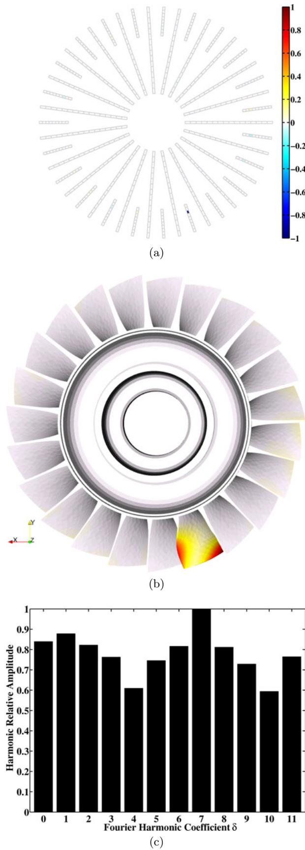
Figure 2.18: (a) Reduced representation of a localized modeshape of the HEBD, (b) its recovery to the full disk and (c) its harmonic content
