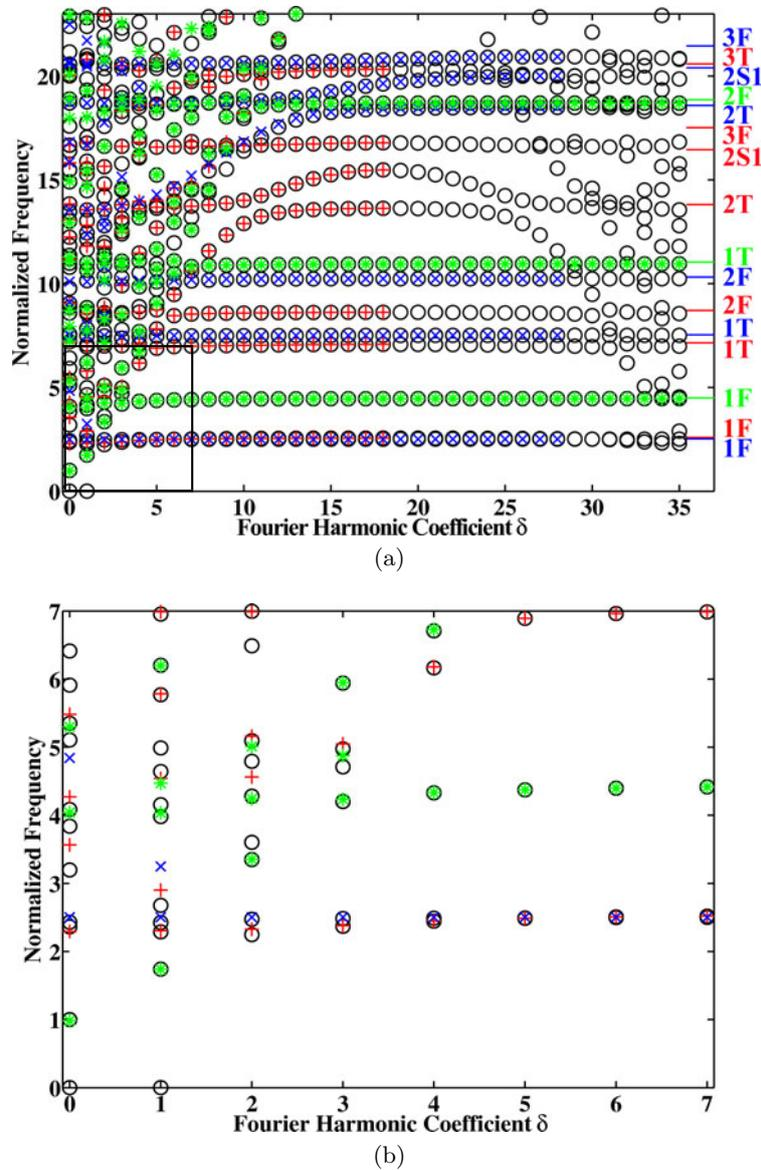
Figure 2.28: (a) Full and (b) zoomed normalized frequencies of the mono-harmonic eigensolutions of the 3SHP model (○) and the modes of disk  $\mathcal{D}^1$  (+), disk  $\mathcal{D}^2$  (×) and disk  $\mathcal{D}^3$  (\*) in free-fix, fix-fix and fix-free condition — (—), (—) and (—) are accumulations
