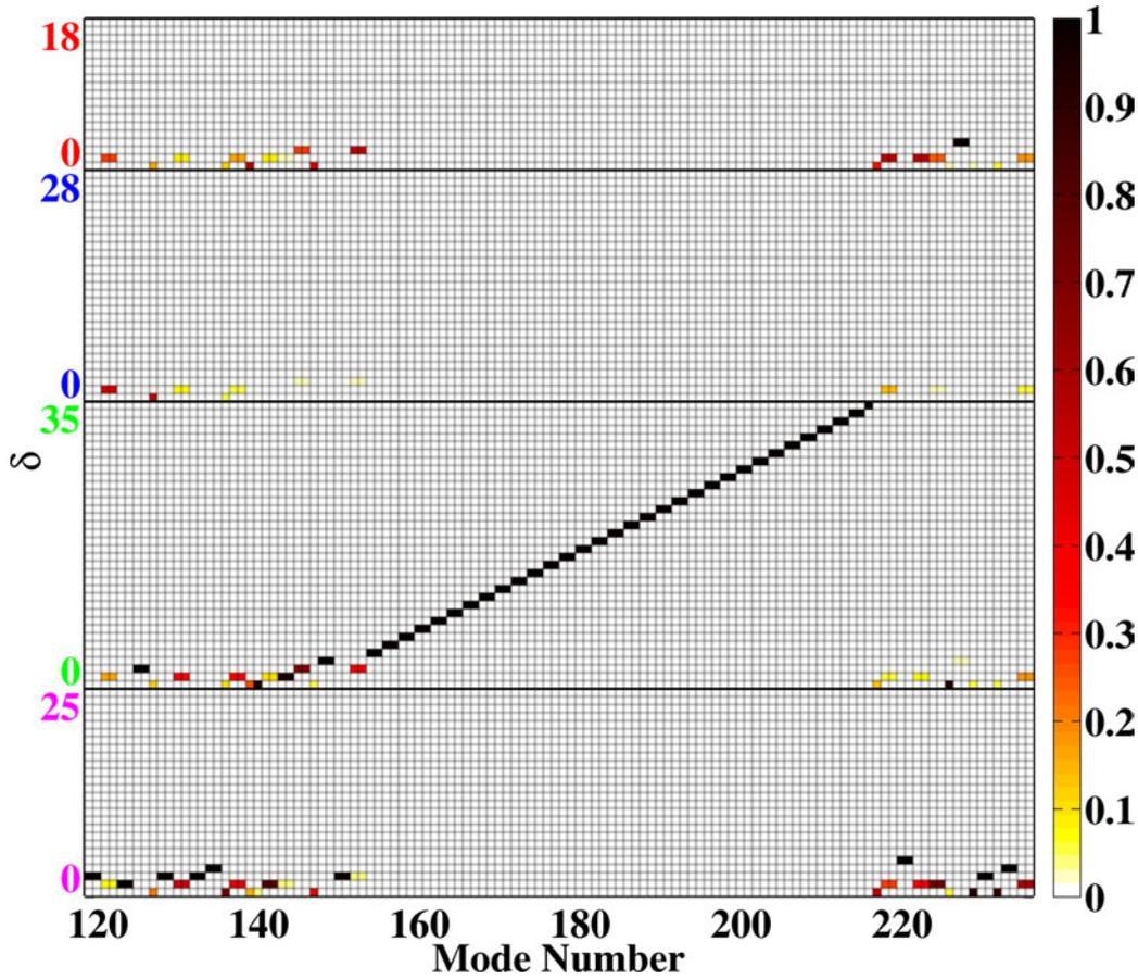
Figure 2.49: Fraction of strain energy by spatial harmonic for the generalized modes in the frequency band  $[2.90, 6.44]$  relative to (from top to bottom)  $\mathcal{D}^1$ ,  $\mathcal{D}^2$ ,  $\mathcal{D}^3$  and  $\mathcal{D}^4$  [FSHP]
