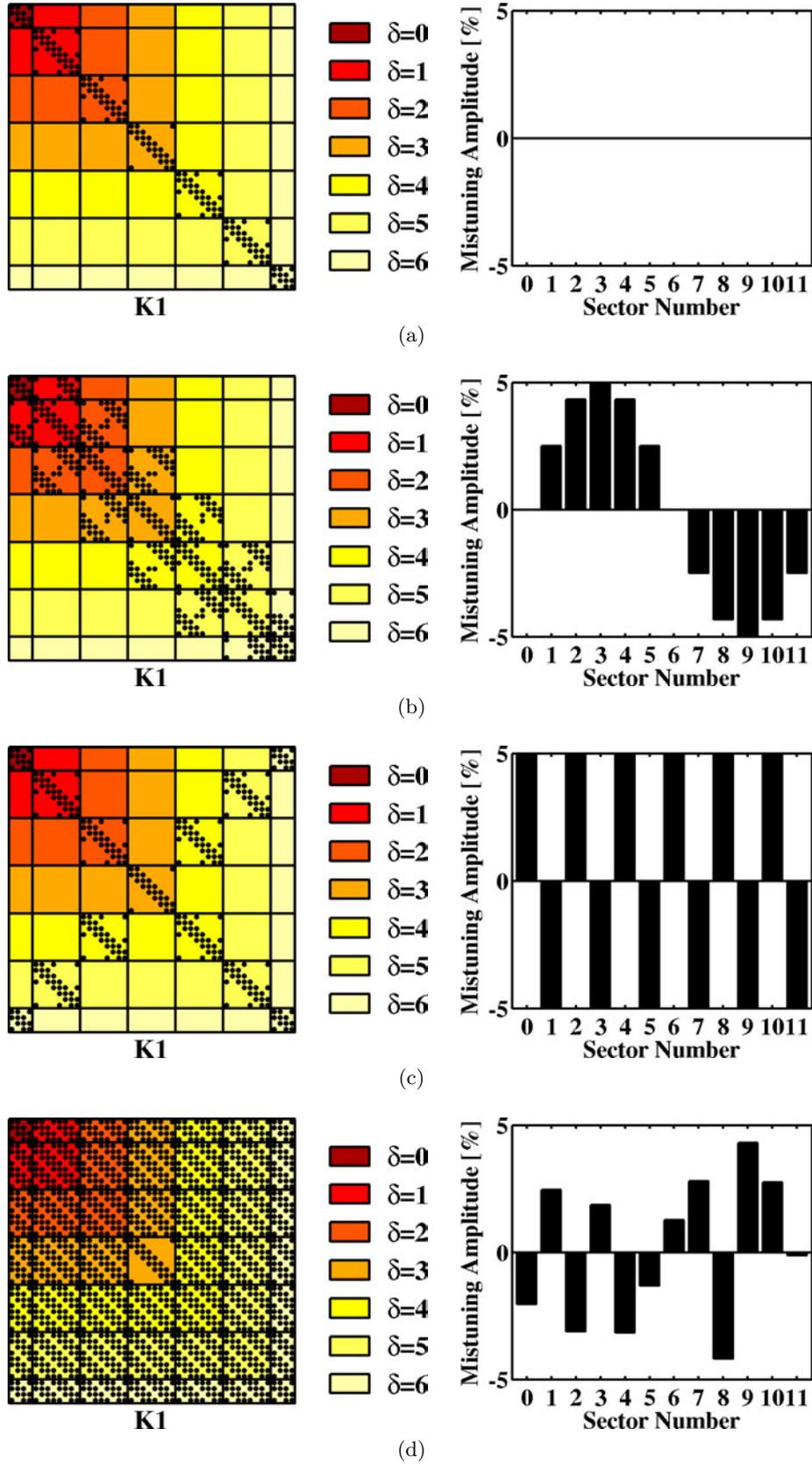
Figure 1.11: Projected stiffness matrix  $[\hat{K} + \Delta\hat{K}]$  of a lumped disk with 12 sectors when (a) tuned and with (b) sine harmonic mistuning with  $\zeta = 1$ , (c) alternate mistuning (cosine harmonic mistuning with  $\zeta = 6$ ) and (d) random mistuning.
