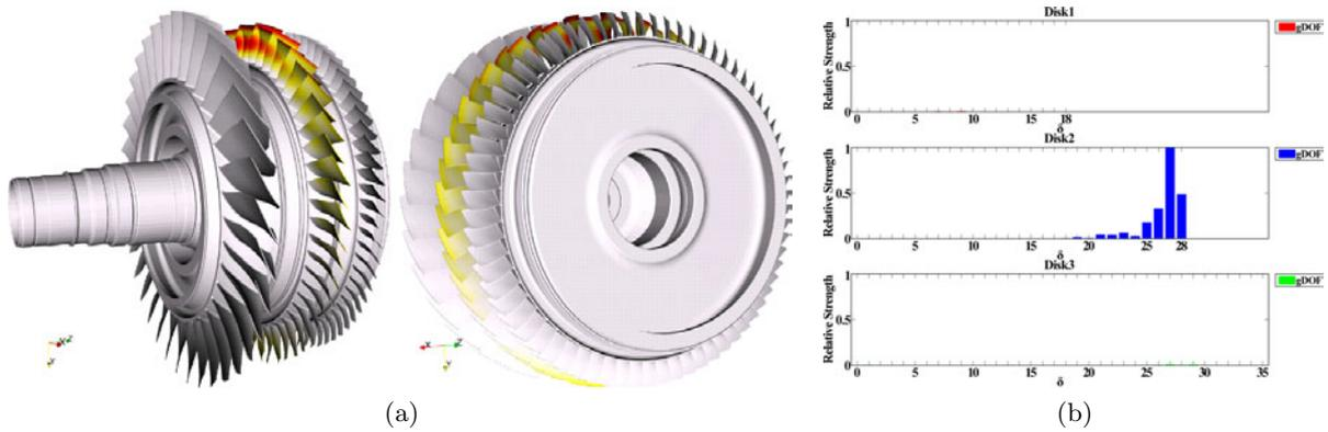
Figure 2.37: Restored mode at  $f = 10.23$  localized to disk  $\mathcal{D}^2$ : (a) modeshape and (b) spatial harmonic content for disks (■)  $\mathcal{D}^1$ , (■)  $\mathcal{D}^2$  and (■)  $\mathcal{D}^3$  [3SHP]
