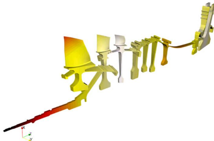
Figure 2.43: Global bending with  $\delta = 1$  at  $f = 1.57$  [FSHP]
