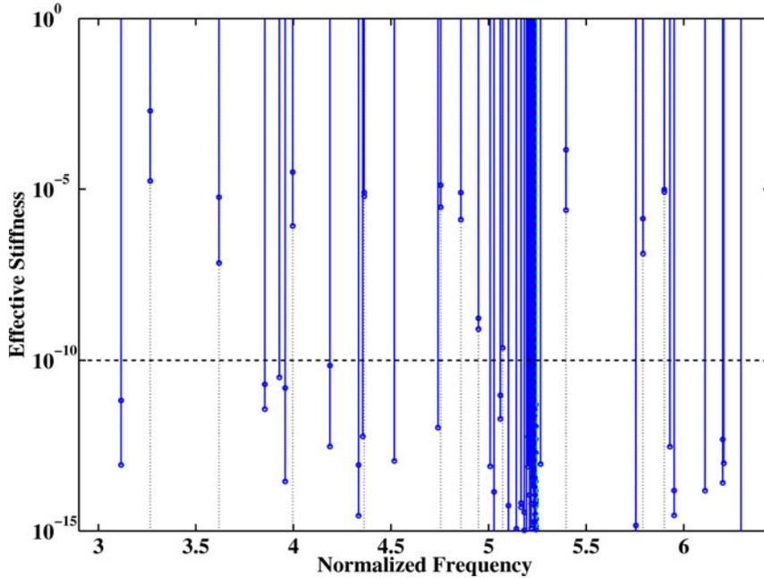
Figure 2.62: Effective stiffness ratios of the generalized modes for the first single DOF load: ( $\dots$ ) assumed controllable modes and ( $- -$ ) 1F accumulation frequency of disk  $\mathcal{D}^3$  [FSHP]
