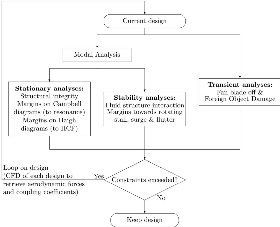
Figure 6: Flowchart of the structural design process
