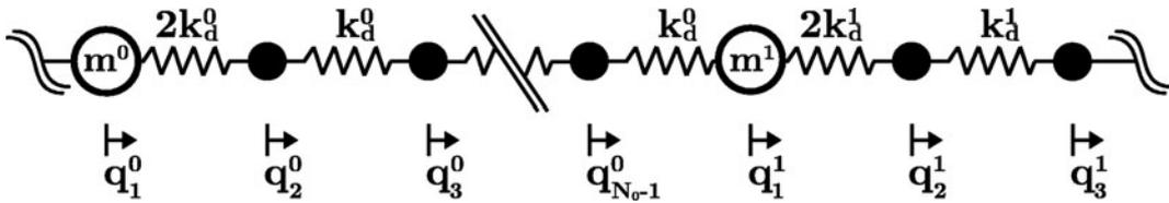
Figure 1.9: Lumped model of a single mistuned disk
