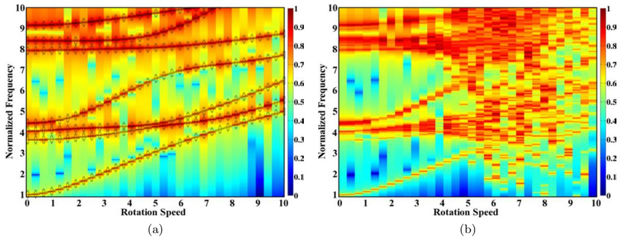
Figure 3.10: (a) Tuned response (with reference Campbell) and (b) mistuned response to a  $\delta = 1$  excitation vs.  $\Omega$  — The color bars refer to the normalized amplitude of the response [HEBD]
