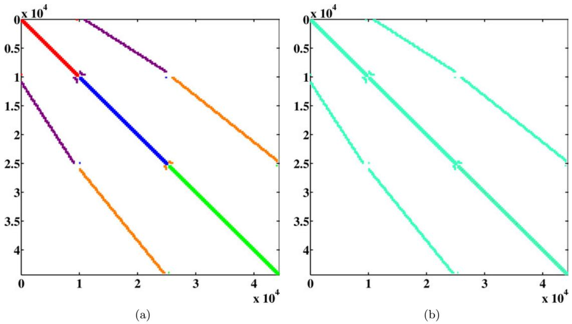
Figure 2.33: Reduced stiffness matrix  $[K_M]$  of the 3SHP model (a) global shape: (■) blocks of disk  $\mathcal{D}^1$ , (■) blocks of disk  $\mathcal{D}^2$ , (■) blocks of disk  $\mathcal{D}^3$ , (■) blocks of ring  $\mathcal{R}^{12}$ , (■) blocks of ring  $\mathcal{R}^{23}$  and (b) actual matrix
