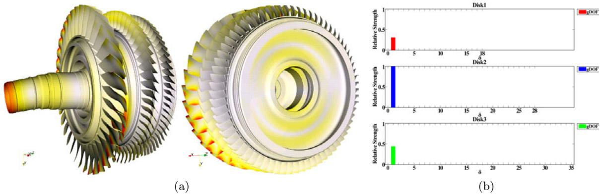
Figure 2.38: Restored mode at  $f = 15.89$  with strong coupling: (a) modeshape and (b) spatial harmonic content for disks (■)  $\mathcal{D}^1$ , (■)  $\mathcal{D}^2$  and (■)  $\mathcal{D}^3$  [3SHP]
