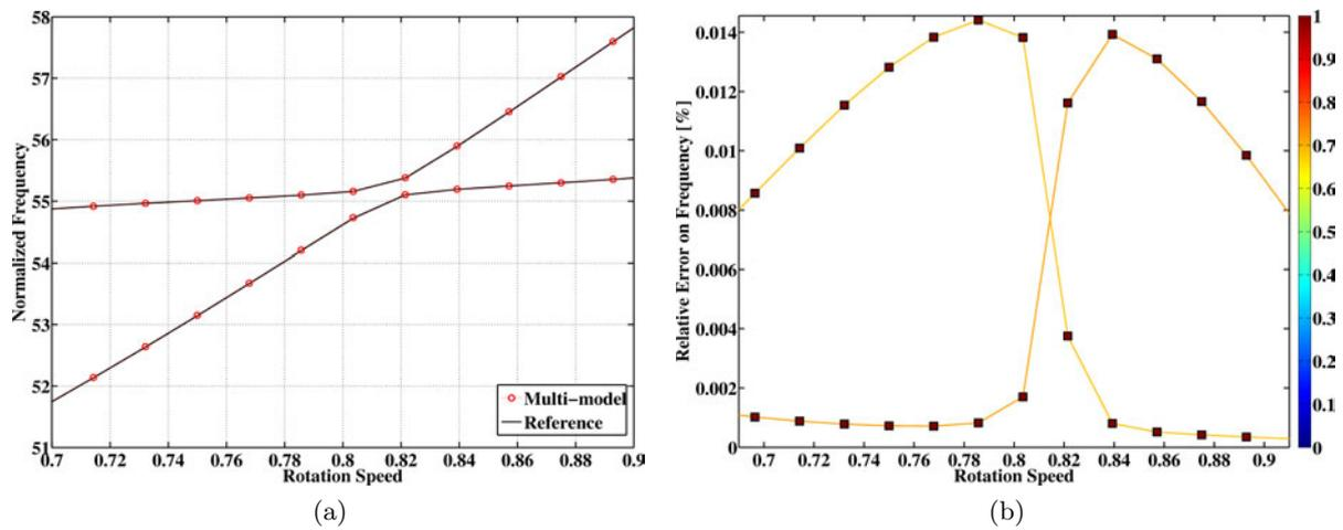
Figure 3.14: (a) Campbell diagram and (b) relative error on frequency and modeshape correlation in the vicinity of the frequency veering event that occurs around  $\Omega = 0.81$  between modes 22 and 23 — The color bar refers to the modeshape correlation [BB]
