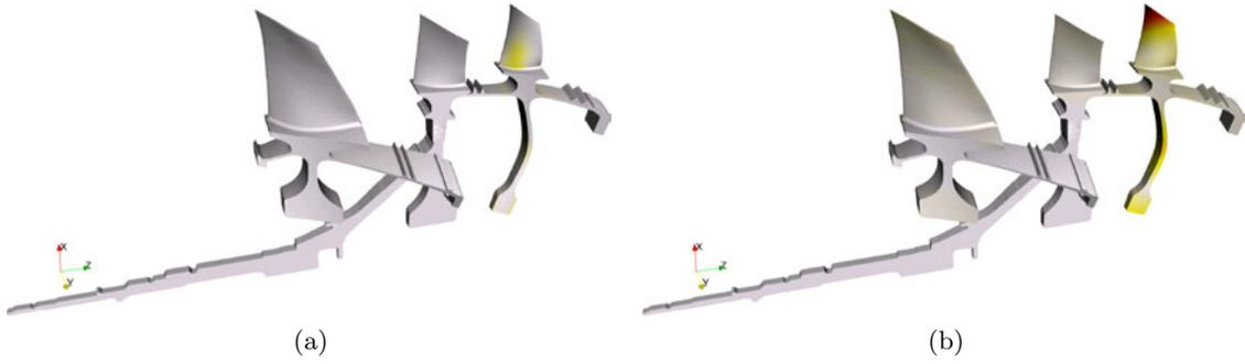
Figure 2.32: Mono-harmonic eigensolution localized to disk  $\mathcal{D}^3$  with  $\delta = 0$  at  $f = 5.35$ : (a) amplitude of the displacement and (b) density of strain energy — Blade shape is 1F [3SHP]
