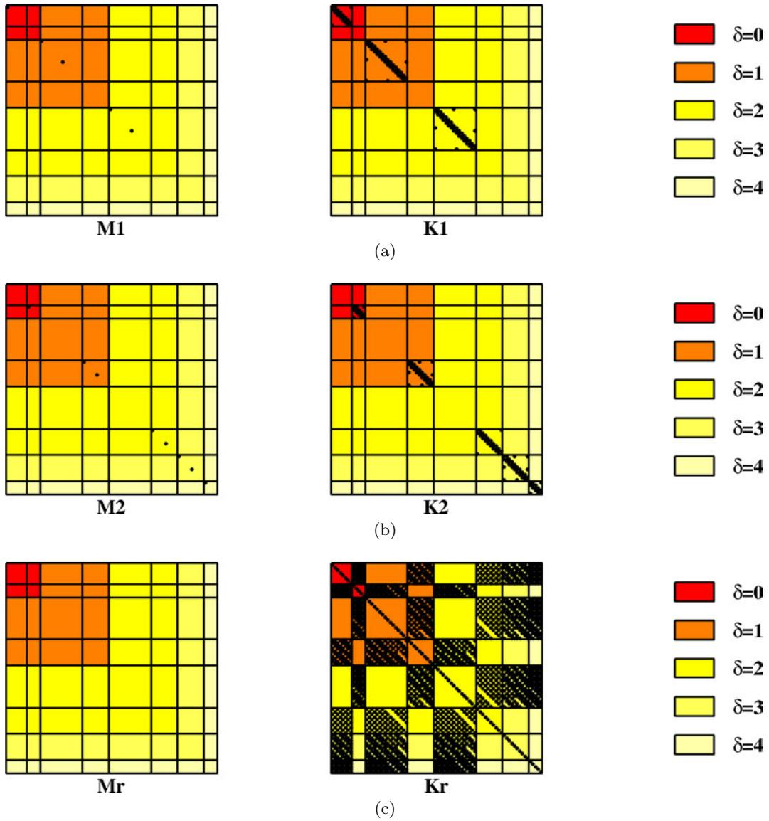
Figure 1.16: Projected matrices of an assembly of disks with 5 and 8 sectors respectively: (a) matrices of disk  $\mathcal{D}^1$ , (b) matrices of disk  $\mathcal{D}^2$  and (c) matrices of ring  $\mathcal{R}$
