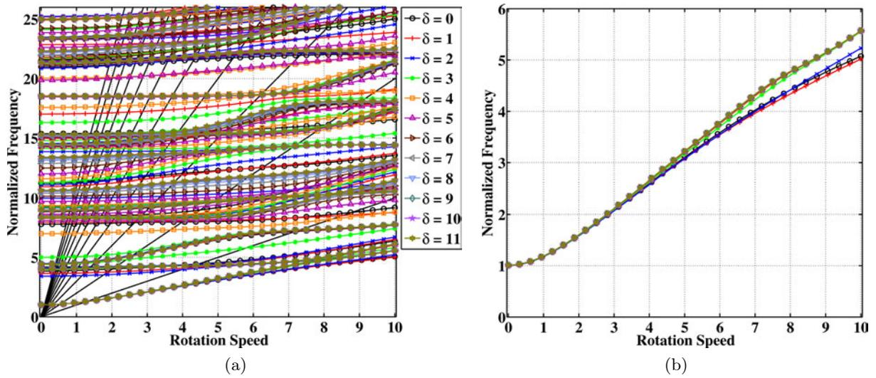
Figure 3.5: Campbell diagram of mono-harmonic modes for  $\delta \in \llbracket 0, \rrbracket 11$  (a) for all modes (with engine orders 1 to 11 in the background) and (b) for the 1F family of modes [HEBD]
