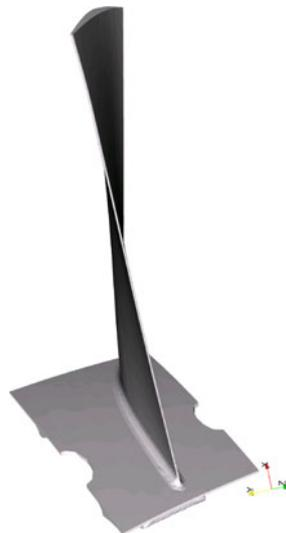
Figure 3.11: Geometry of the booster blade
