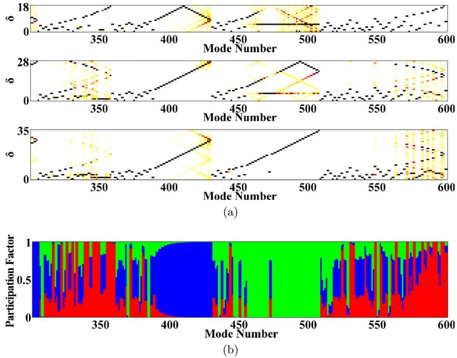
Figure 2.35: Generalized modes 301 to 600 ( $f \in [7.52, 13.74]$ ): (a) Spatial harmonic content and (b) participation factor in strain energy for disks ( $\blacksquare$   $\mathcal{D}^1$ , ( $\blacksquare$   $\mathcal{D}^2$  and ( $\blacksquare$   $\mathcal{D}^3$  [3SHP]
