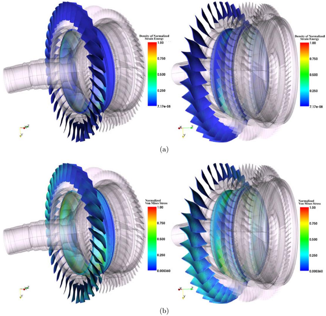
Figure 2.41: Partial post-processing of the generalized mode at  $f = 15.89$  on disk  $\mathcal{D}^1$ : (a) normalized density of strain energy and (b) normalized distribution of Von Mises stress [3SHP]
