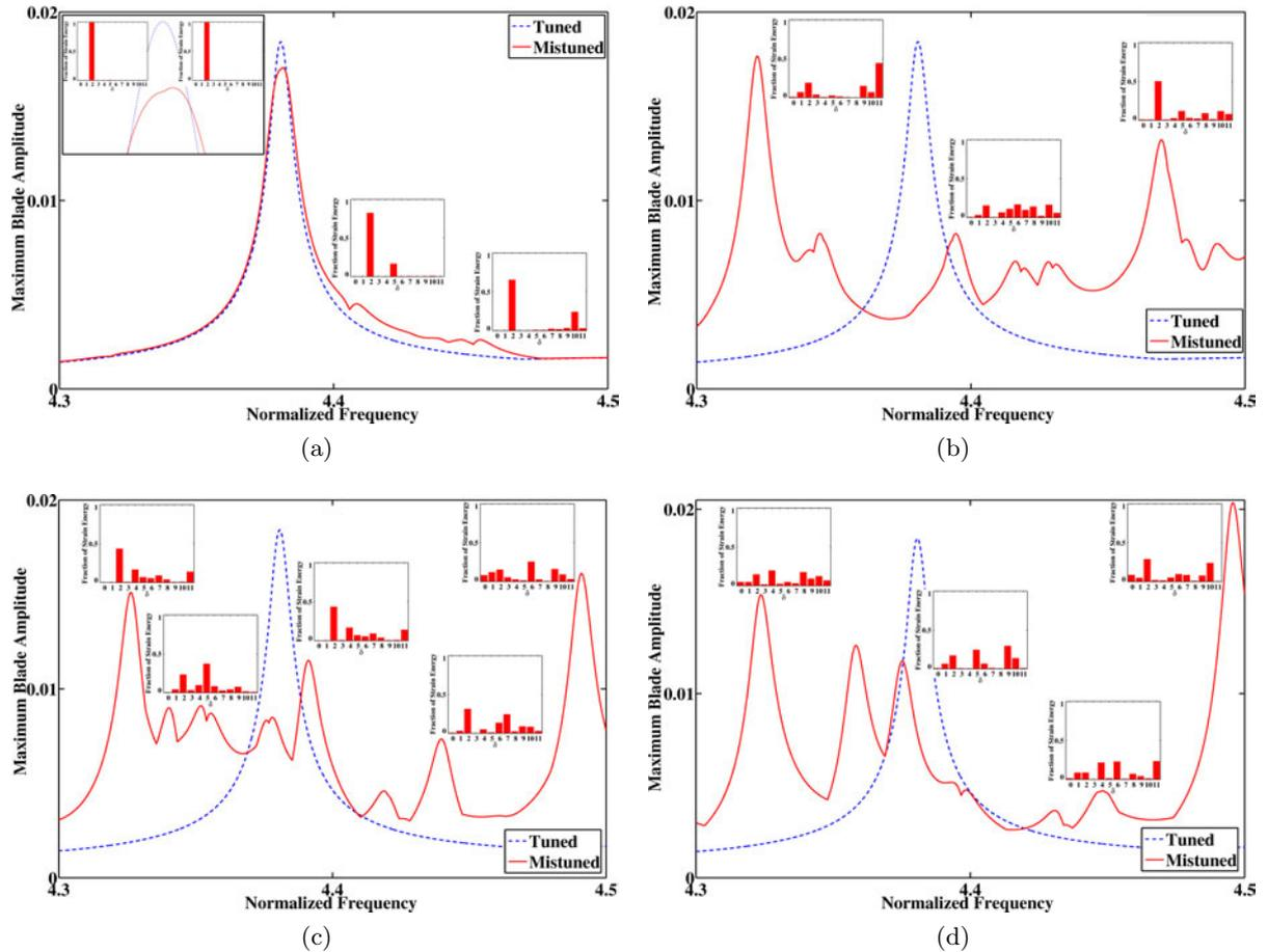
Figure 1.10: Tuned and mistuned responses of a sample disk with 23 blades to an excitation with  $\delta = 2$  and DFT of the response at some peaks when the distribution has a standard deviation of (a) 0.5%, (b) 5%, (c) 10% and (d) 20%
