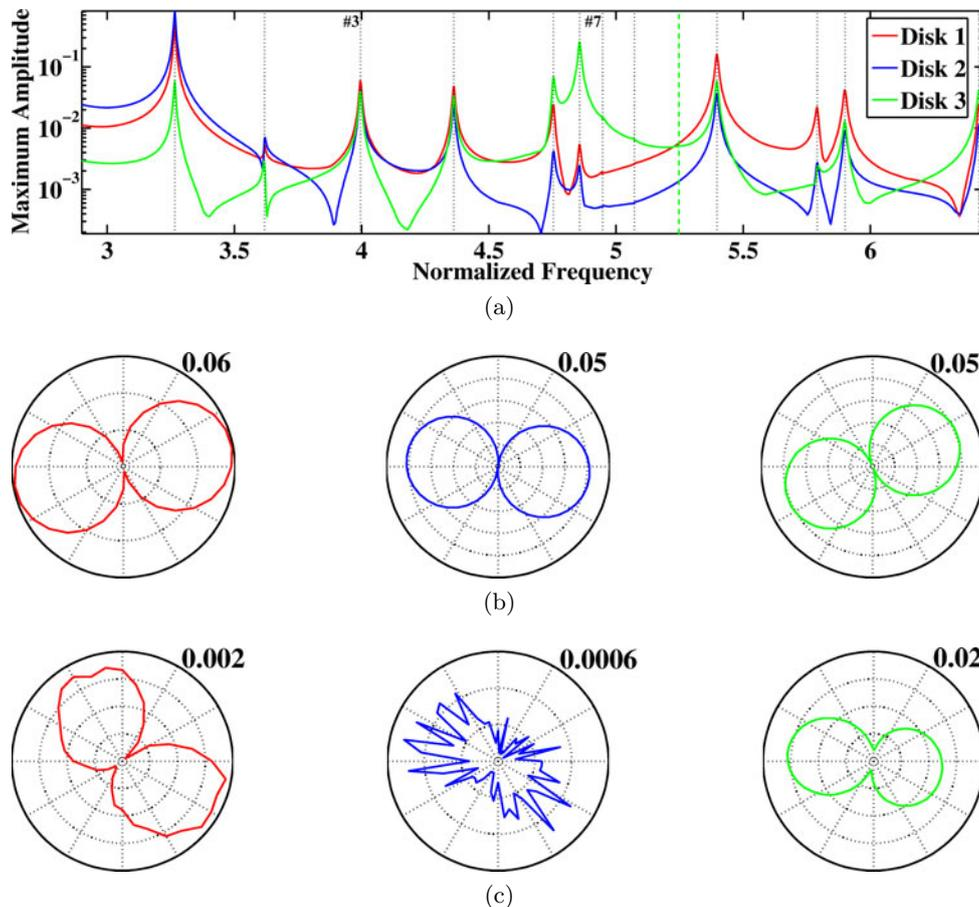
Figure 2.66: Measured displacement at sensors: (a) considered resonances and amplitudes at resonance (b) 3 and (c) 7 for (—) disk  $\mathcal{D}^1$ , and (—) disk  $\mathcal{D}^2$  and (—) disk  $\mathcal{D}^3$  [FSHP]
