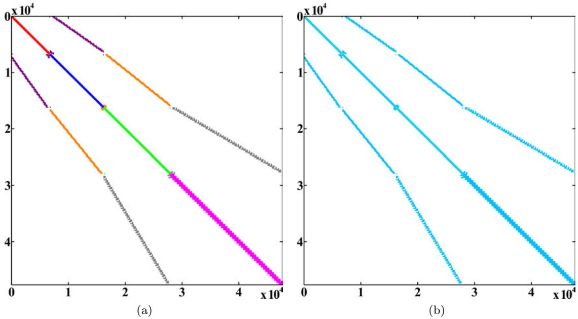
Figure 2.47: Reduced stiffness matrix  $[K_M]$  of the FSHP model (a) global shape: (■) blocks of disk  $\mathcal{D}^1$ , (■) blocks of disk  $\mathcal{D}^2$ , (■) blocks of disk  $\mathcal{D}^3$ , (■) blocks of disk  $\mathcal{D}^4$ , (■) blocks of ring  $\mathcal{R}^{12}$ , (■) blocks of ring  $\mathcal{R}^{23}$  and (■) blocks of ring  $\mathcal{R}^{34}$  and (b) actual matrix
