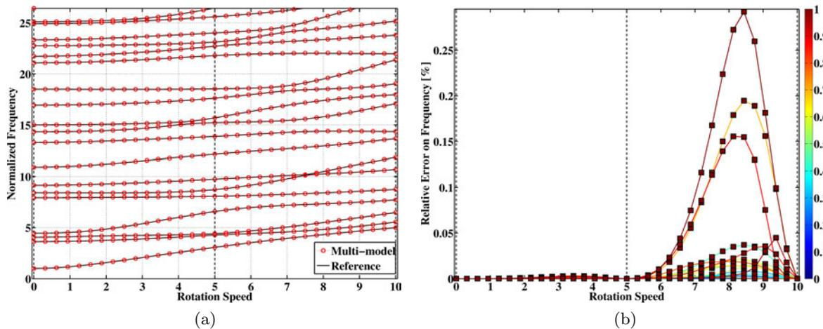
Figure 3.6: (a) Campbell diagram for  $\delta = 1$  and (b) relative error on frequency for a multi-model basis built at  $\Omega \in \{0, 5, 10\}$  — The color bar refers to the modeshape correlation [HEBD]
