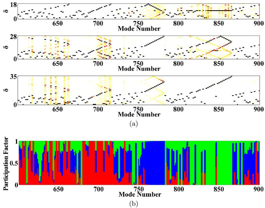
Figure 2.36: Generalized modes 601 to 900 ( $f \in [13.76, 19.57]$ ): (a) Spatial harmonic content and (b) participation factor in strain energy for disks ( $\blacksquare$   $\mathcal{D}^1$ , ( $\blacksquare$   $\mathcal{D}^2$  and ( $\blacksquare$   $\mathcal{D}^3$  [3SHP]
