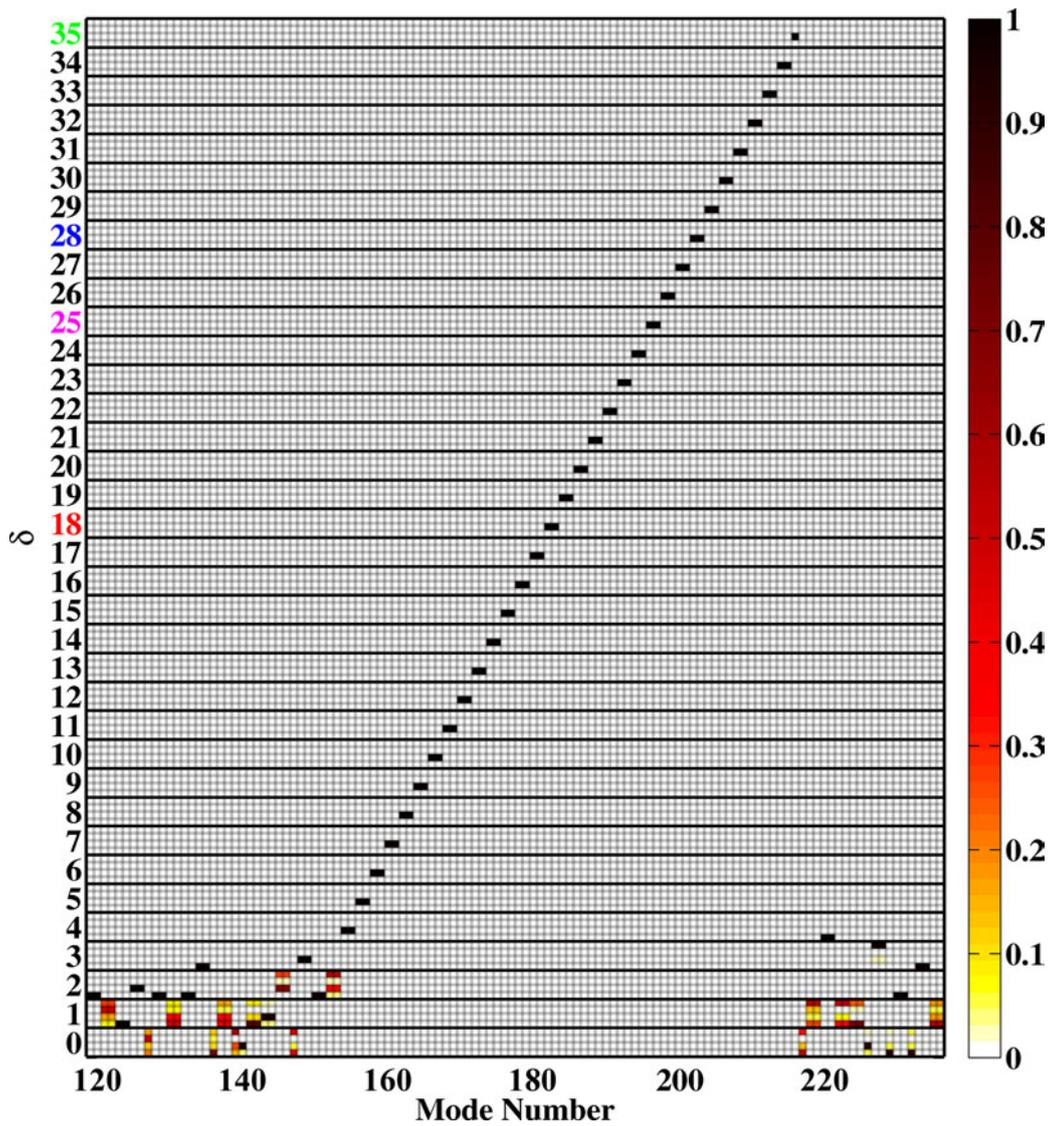
Figure 2.50: Fraction of strain energy by spatial harmonic for the generalized modes in the frequency band [2.90, 6.44] relative to (from top to bottom for each harmonic)  $\mathcal{D}^1$ ,  $\mathcal{D}^2$ ,  $\mathcal{D}^3$  and  $\mathcal{D}^4$  [FSHP]
