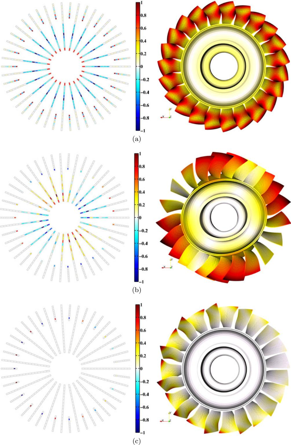
Figure 2.15: Reduced representations of the modeshapes (left) and their recovery to the full HEBD (right) for mono-harmonic modes with: (a)  $\delta = 0$ , (b)  $\delta = 2$  and (c)  $\delta = 11$
