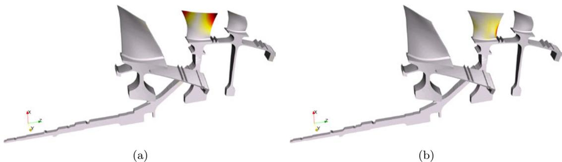
Figure 2.31: Mono-harmonic eigensolution localized to disk  $\mathcal{D}^2$  with  $\delta = 2$  at  $f = 7.47$ : (a) amplitude of the displacement and (b) density of strain energy — Blade shape is 1T [3SHP]
