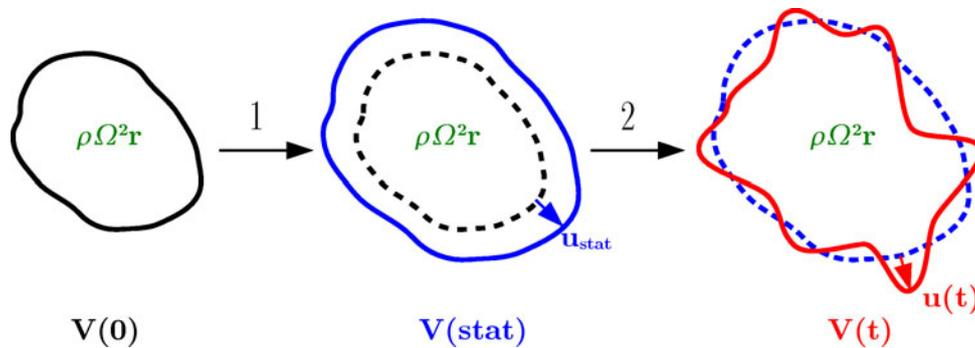
Figure 3.1: The two steps used to compute the response of a structure rotating at a constant speed
