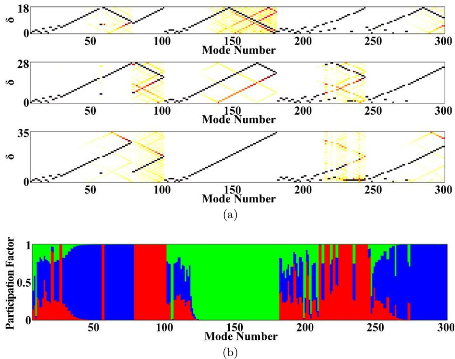
Figure 2.34: Generalized modes 7 to 300 ( $f \in [1, 7.52]$ ): (a) Spatial harmonic content and (b) participation factor in strain energy for disks (■)  $\mathcal{D}^1$ , (■)  $\mathcal{D}^2$  and (■)  $\mathcal{D}^3$  [3SHP]
