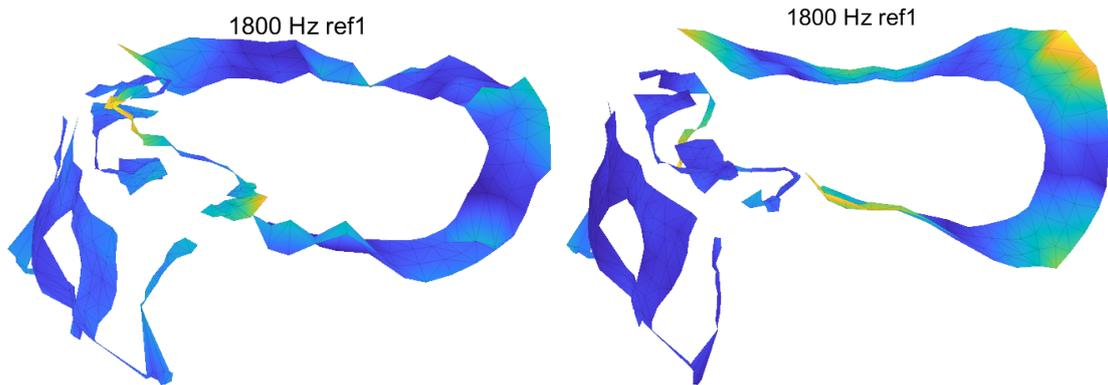
Figure 3.42: ODS extracted from a 3D-SLDV measurement using H1 transmissibility. Left: real part. Right: imaginary part. Color indicates displacement normal to the disk.
