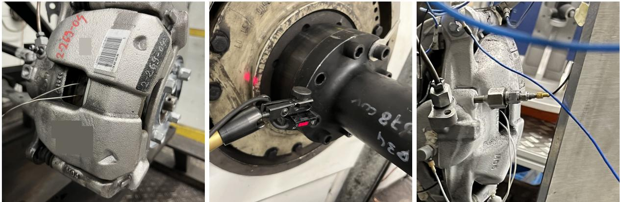
Figure 3.5: Placement of sensors in the test bench Left: pad temperature sensor. Center: tachometer. Right: pressure sensor.
