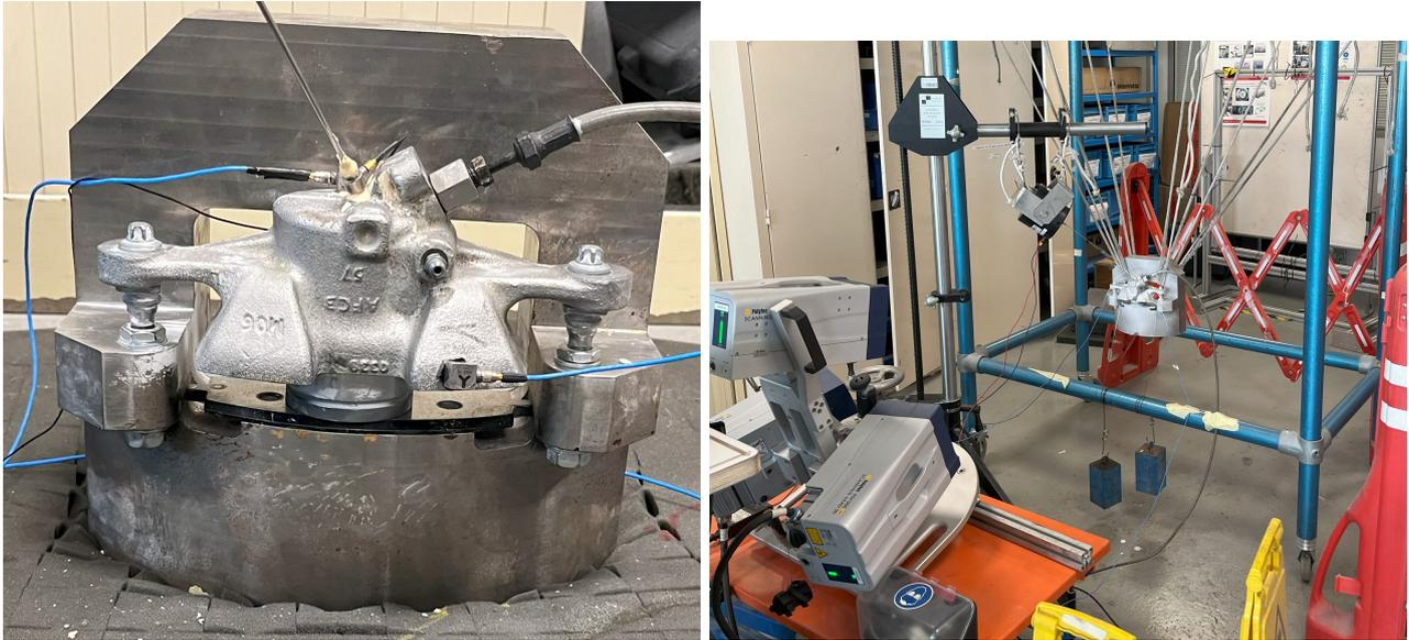
Figure 2.19: Second design of the contact test bench on the ground (left) and suspended (right)
