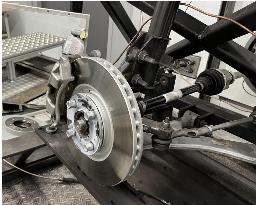
Figure 3.4: Brake system mounted in the test bench, 2023 setup.
