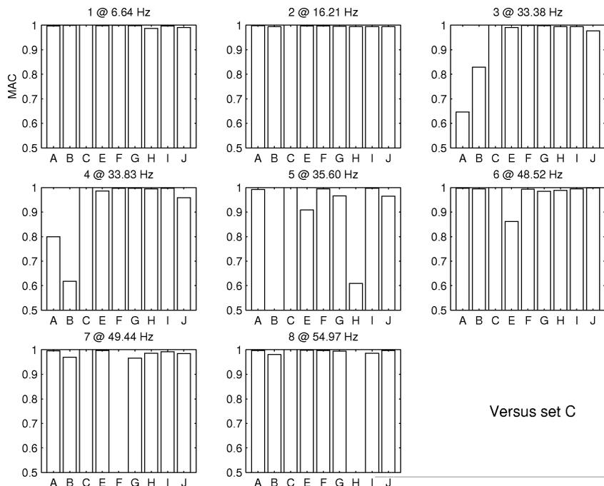
Figure 12. Diagonal MAC values for comparison of different test modeshapes with those of test C.
