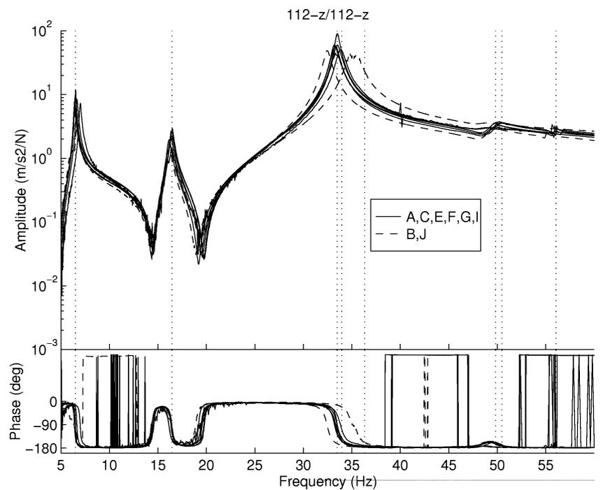
Figure 6. Collocated transfer function at left drum (112z).
