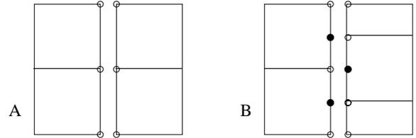
Fig. 1: Continuity constraints  $c_{int}$  can be built by enforcing continuity of displacements at nodes of the elements  $\circ$  as well as intermediate nodes  $\bullet$ .
