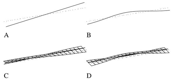
Fig. 4: A-B: interface deformations linked to the interpolation functions of standard beam elements. C-D: interface deformations linked to a local model.
