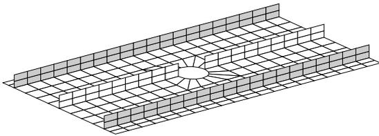
Fig. 3: Stiffened panel with a hole. The components are a main piece (skin and middle stiffener) and two edge stiffeners (shaded in gray).
